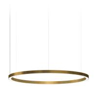
Suspension lighting fixture for interiors, with direct light emission. Bended extruded aluminium structure in white, black or mat brass polyacrylic paint. Extruded polycarbonate diffuser with opaline finish. Suspension kit with griplocks and 2m (78,7") long steel cables. 2,2m (86,6") long power cable in transparent PVC. Power canopy with pickled sheet metal ceiling bracket and covering in white polyacrylic paint.
